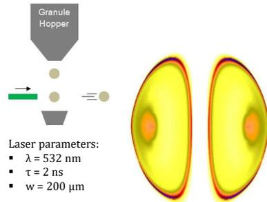
Fig. 2: Schematic of granule laser-injection device.
