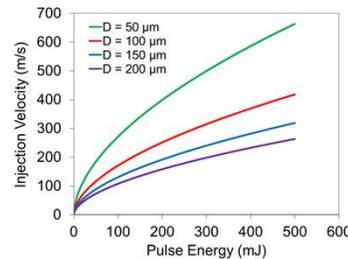
Fig. 3: Injection velocities for Li granules of various size.
