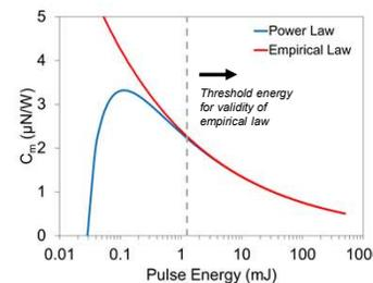
Fig. 4: Impulse coupling as predicted by power and empirical scaling laws [1].
